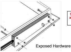
Supplied countersink bushings are neccessary to reduce stress when platform is in motion.
