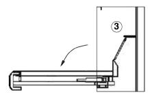
Lower door and install the mattress on the bed frame in preperation for adjusting the balance of the platform.
