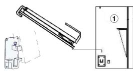
Lift door platform and bed frame on a 45° angle to clear all obstructions and lower the assembly into place with the square axels in the mount plate saddles in the cabinet.
