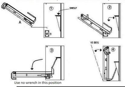
Adjust tension with bed platform at 15° from vertical and with mattress inplace Tighten tension screws on each side of bed progressively to maintain balance
