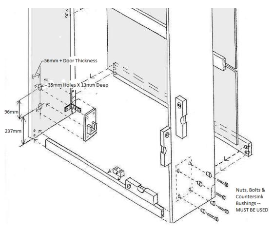
Install Platform into Cabinet with foot elevated to at least 45°. With Platform 15° from vertically closed use a 24mm Socket to adjust tension
